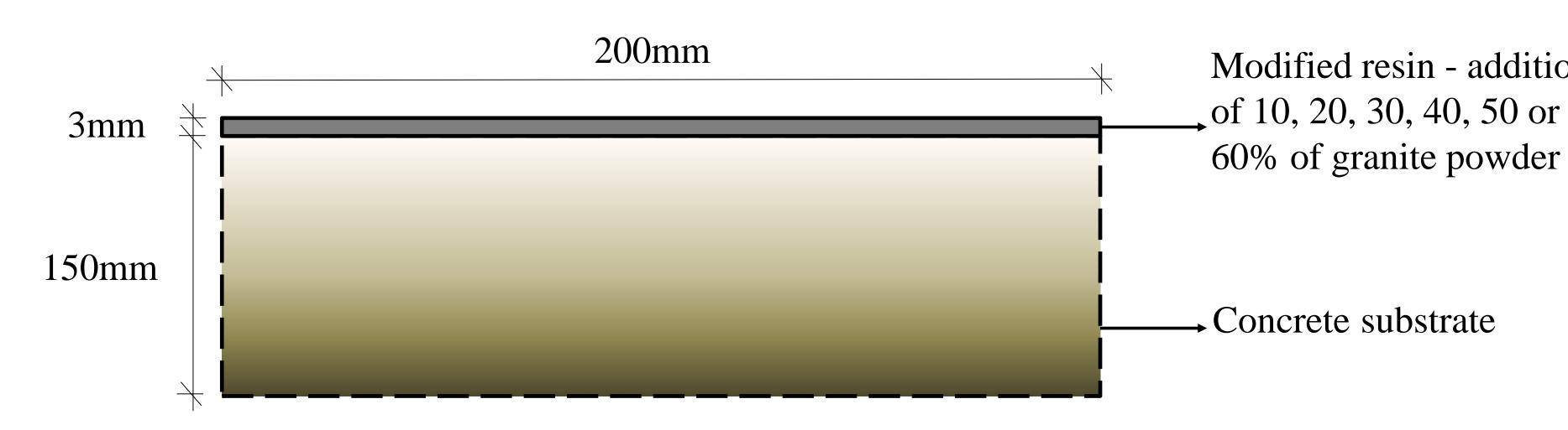
The test began with the preparation of the substrate, made of C30 / 37 concrete, S3 consistency, supplied by a specialized company. After its full hardening, the surface was ground and degreased. The resin used consisted of two components: A and B. After the first component was measured out, a measured amount of granite powder was added. After mixing, component B was added and mixed again. The modified resin was then applied to the substrate to obtain a 3mm layer.
